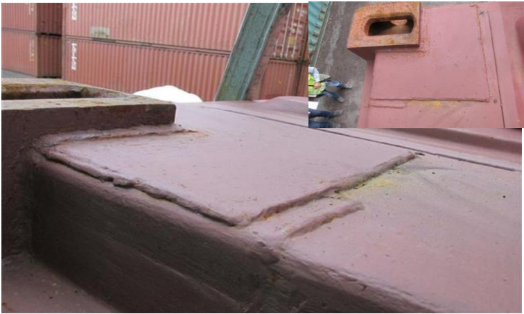
Proper replacement of the corner protection plate after installation of insert on the front header.
