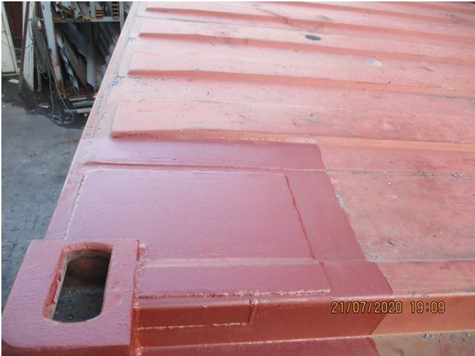
Proper replacement of the corner protection plate after installation of insert on the front header.
